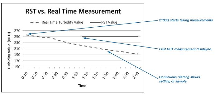
Although the sample continuously settles out of solution, the RST calculated value does not change. No more guessing and no more replicate runs
