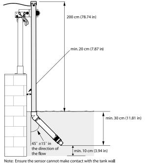
sensor cannot make contact with the tank wall
