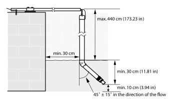
Note: Ensure the sensor cannot make contact with the tank wall
